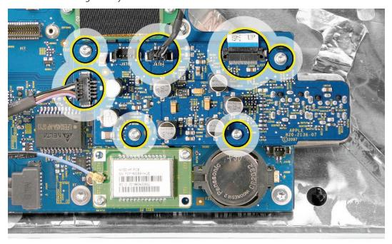
3. Lift the audio board off the logic board.
